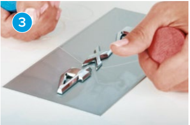
Position the fishing line between the painted metal and the attached part while the materials are still hot.
