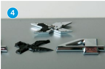
Start sawing through the tape with the fishing line until the part is detached from the metal sheet.
