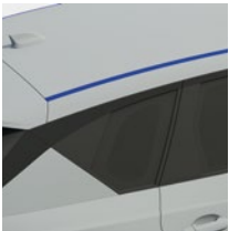
Roof ditch trim
