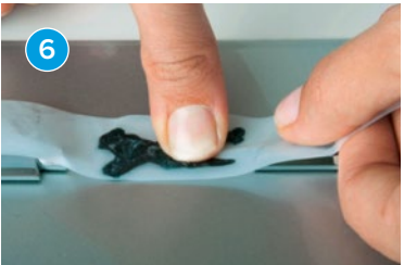
Ensure that the film is completely bonded to the adhesive residue by pressing it with your thumb. As the residue might be still hot, wear protective gloves.
