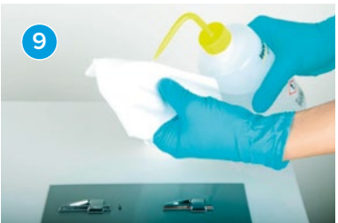
Finish the cleaning process by wiping the surface with isopropyl alcohol and dry it with a lint-free cloth before attaching the new part.
